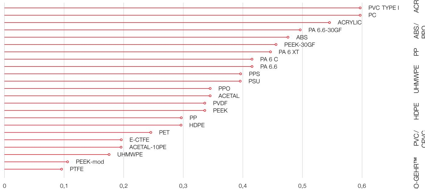
plastic/steel 16 MnCr 5; Rt = 2 mmM, surface pressure = 0.05 MPa, sliding speed = 0,6 m/s; surface temperature = 140 °F
