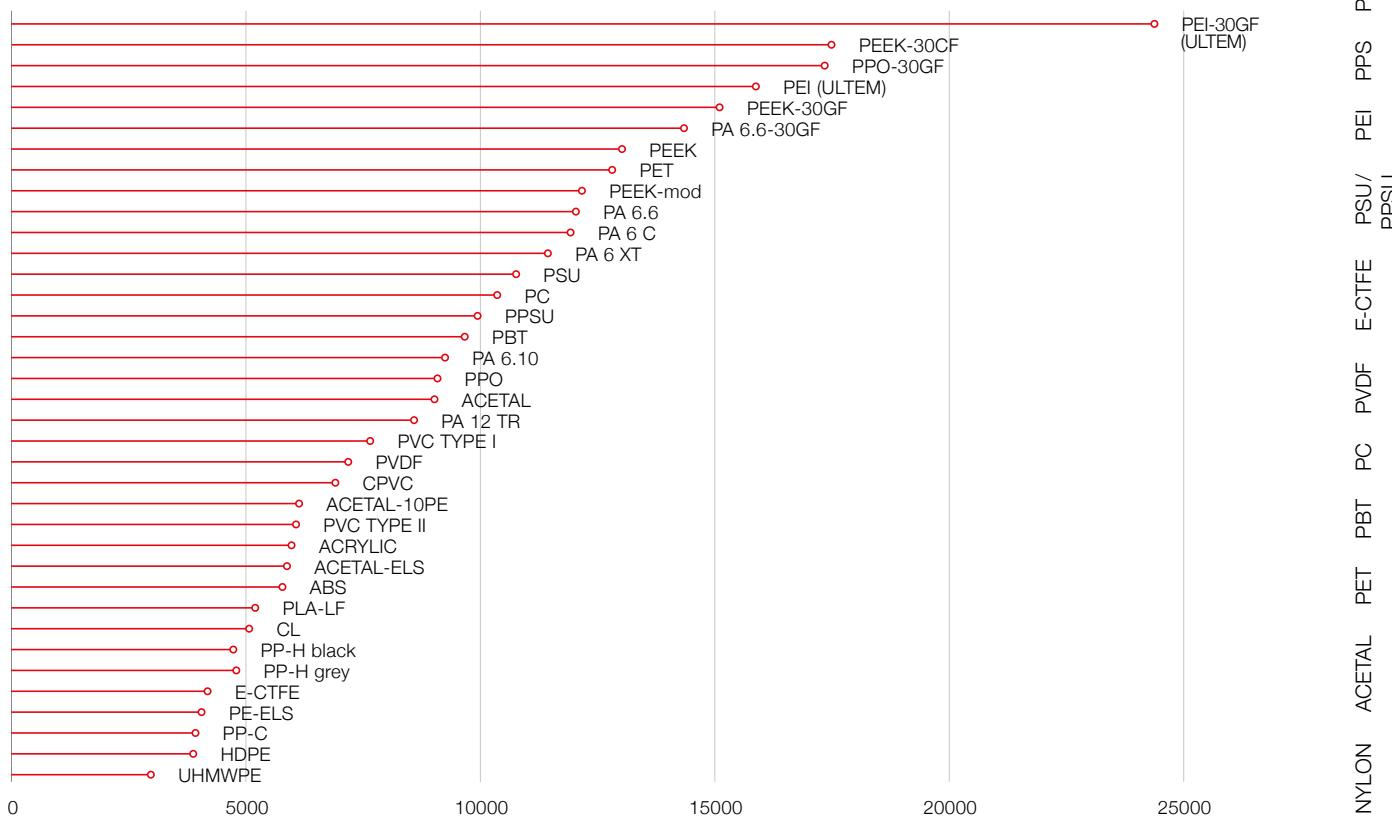
**Modulus of elasticity versus tensile strength at yield (psi)**
