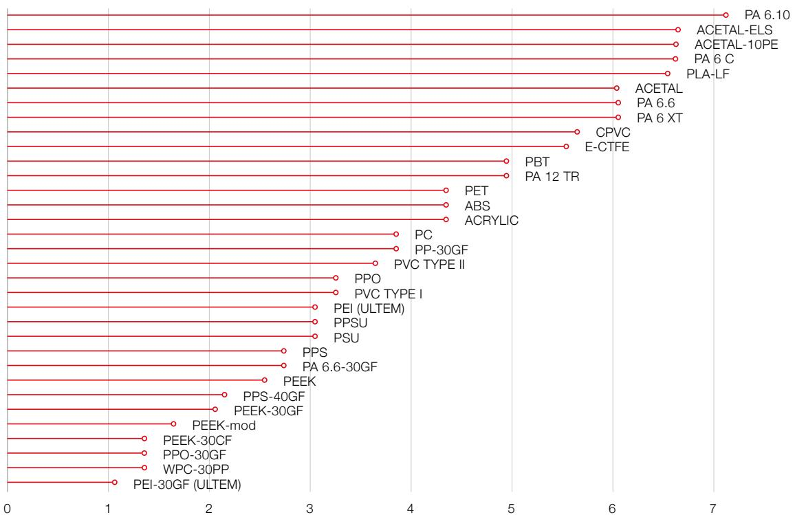
**Linear expansion of the different materials in relation to the absorption of humidity**
